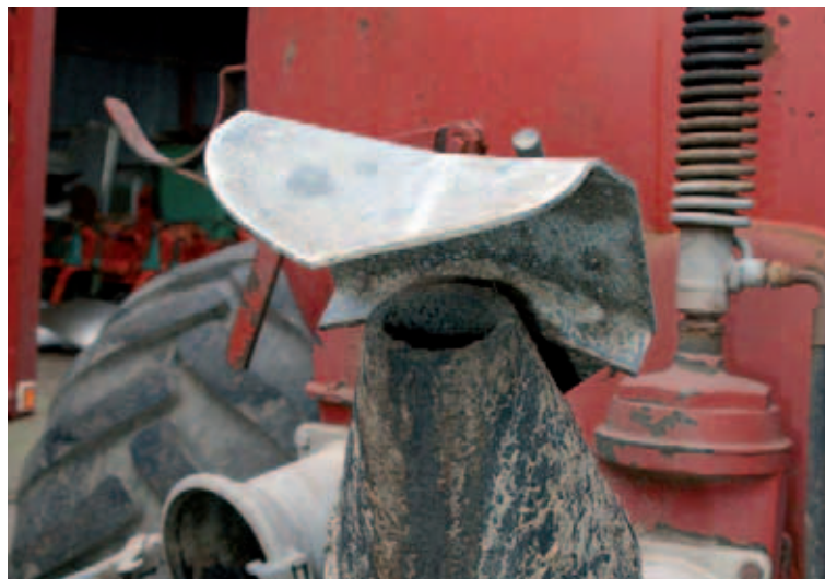
Photo 20: Inverted splashplate slurry spreading
